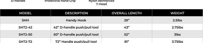
Ratings: Load Testing - Static Pull = 400 lbs. / Compression = 600 lbs. Our tools are not lifting/load bearing tools, SWL cert not required. Major components tested to ASTM standards. Seeking NOPSA (AU) Review. Made in USA.
